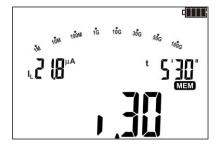
The value of leakage current I<sub>L</sub> measured in time t=5'30'. Symbol Jundicates the selected time interval, in which the leakage current value was recorded.
