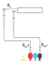
Connect test leads according to the drawing.
