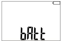
The battery pack is fully discharged,
