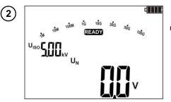
The meter indicates readiness for measurement with increasing voltage.
