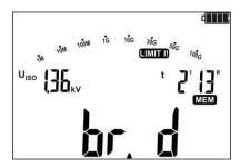
If the electric resistance strength of the tested insulation is exceeded and the puncture occurs, the main field of the display will show message br. d - breakdown.
