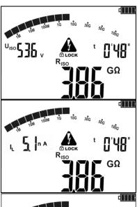
View of the screen during measurement. DLOCK means that the measurement was started with ENTER button or by pressing and holding START but-
