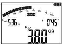
After the measurement is completed or stopped, read the result. The results of all completed measurements will be displayed (even when the measurement was interrupted)
